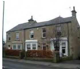
(14) Earlwood House and Oakdale House Early 20 th century semi-detached properties. Constructed of squared stone to front and modern to rear
